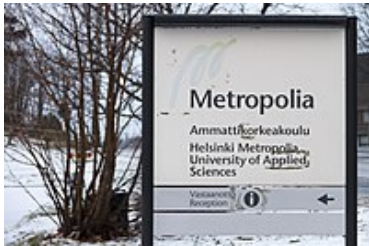
Side of a sign of the University of Applied Sciences oriented towards the southeast where direct sunlight impacting from dawn to afternoon has bleached the red and yellow colors from the logo of the institution.
